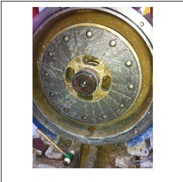
Figure 7 :double disk refiner Factory 1
