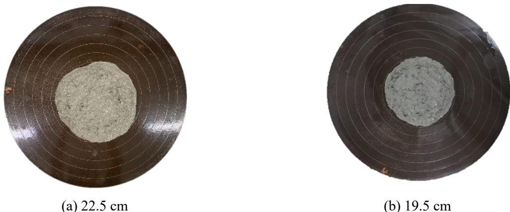
Figure 2 – Flow table test on mixtures of (a) WBC45-0.35 and (b) WBC45-0.30.
