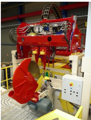
Figures 27, 28 - Eltomatic CVS-16 Wood Wool Machine
