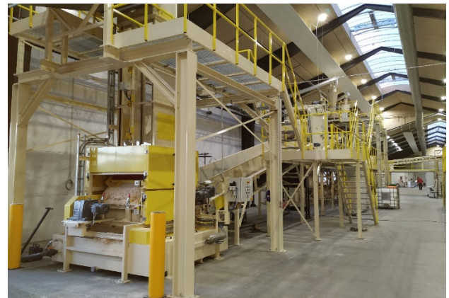
Figure 29 – Dosing and Mixing Group
