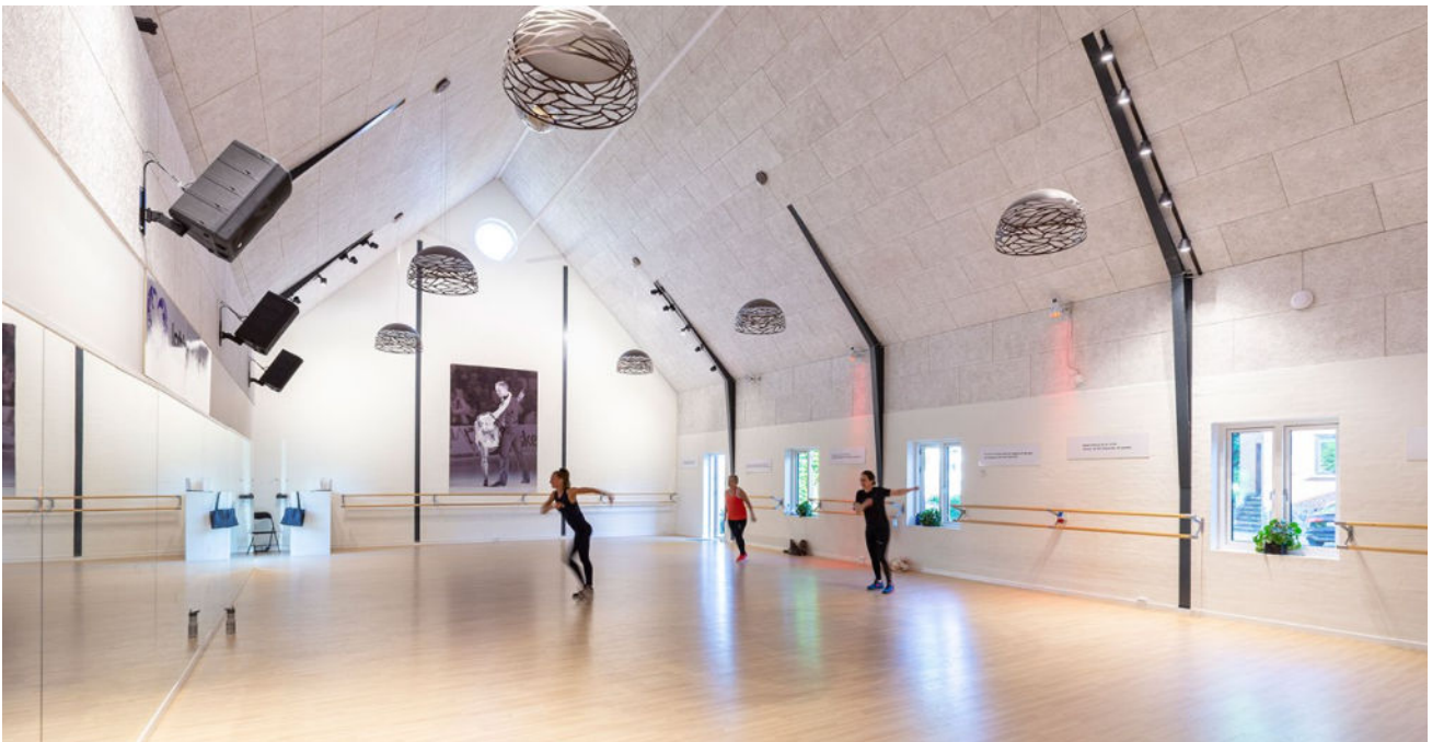
Figure 9, 10, 11 – Acoustic applications of WWCB in various public buildings (Troldekt, Denmark)
