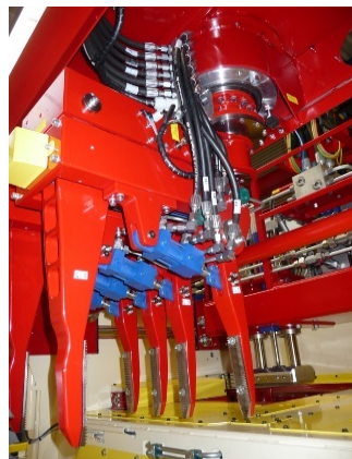
Figures 27, 28 - Eltomatic CVS-16 Wood Wool Machine
