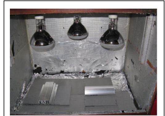
Figure 7 : Interior of the dry UV chamber in which the reference and post treated boards were submitted to accelerated ageing under UV light.
