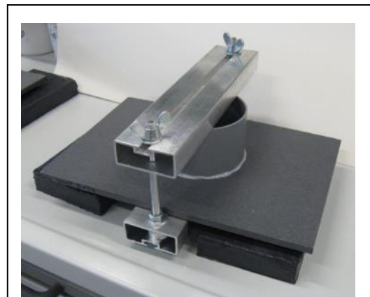
Figure 6 – Illustration of Cobb test.
