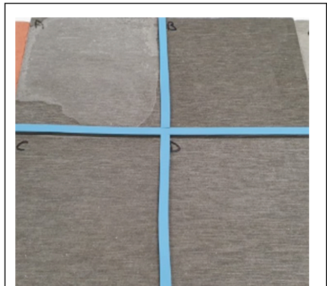
Figure 12: visual observation of reference (A) or treated FC boards (treated with DOWSIL™ IE 6710 emulsion diluted at 10% Active content = B, 15% active content = C and 20% active content = D) after the accelerated efflorescence test
